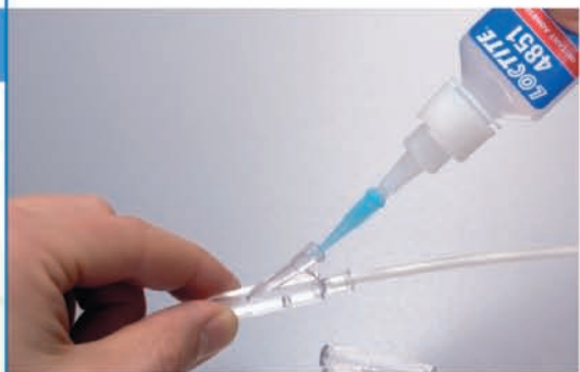
Needle tip adapters used on adhesive bottles, pg. 12
